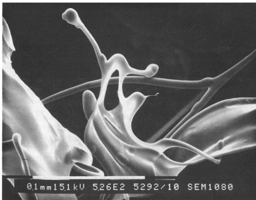
Fig. 7. Scanning electron microscopy of freeze-dried N -carboxybutyl chitosan, showing its film-forming ability ( \times 526 ).
